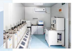
Coalbed methane (gas) content testing mobile laboratory (independent research and development)
