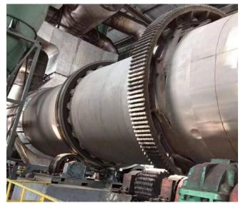
Coal slurry drying set powered by catalytic oxidation system for coal mine gas with methane concentration around 1% to 1.2%.
