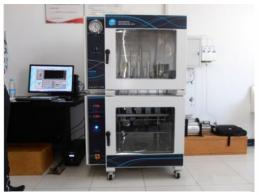
gravimetric adsorption instrument
