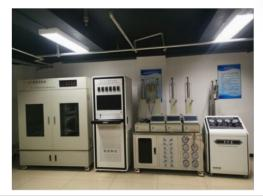
Multi-layered stacked gas reservoir joint development simulator
